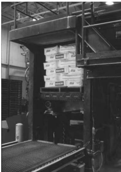
FIGURE 16.1 An autopalletizer for sacks eliminates manual lifting.
