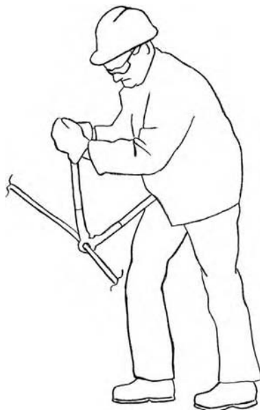
FIGURE 14.B2 Cutting cable, bracing one handle of the manual tool against the hip.
