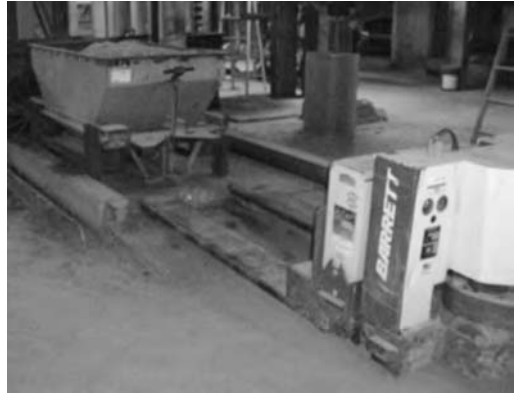
FIGURE 16.18 A heavy-duty-pallet truck used to pick up and transport a wagon.
