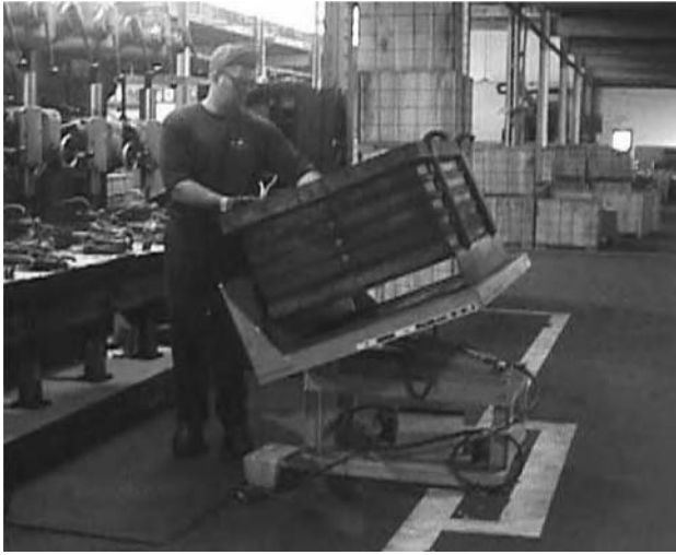
FIGURE 13.2 Lift and tilt table reduces bending by providing easy access to parts.
