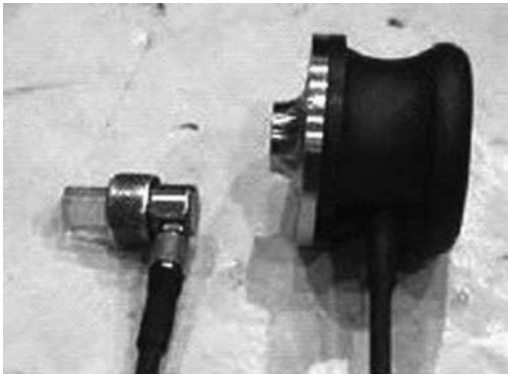
FIGURE 3.17 After: Working with in-house resources, newly designed nylon handles were fabricated. These handles are three times larger, thereby reducing the pinch force. (From Boeing Commercial Airplane Group Seattle, WA 2003 and Zawitz Ben, Ergonomics at Boeing . Ergosolutions magazine July/August 2003. With permission.)
