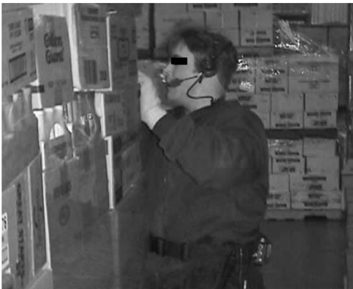
FIGURE 45.25 Headsets, used to direct selectors through their order, freeing both hands for selecting.
