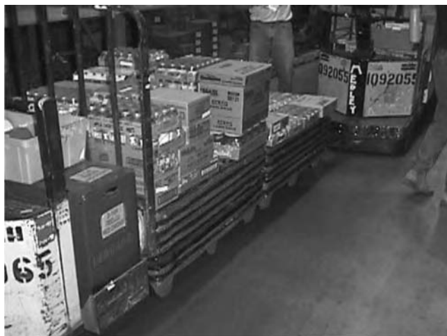
FIGURE 45.21 Stacking of empty pallets on a pallet jack, to raise the initial stacking height of cases and reduce trunk bending.
