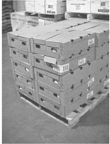
FIGURE 45.8 Handle cut-outs in cases, to ease lifting and carrying.
