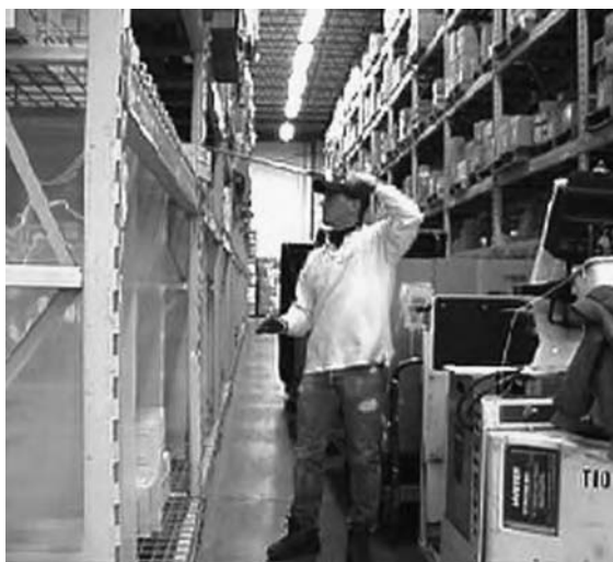
FIGURE 3.12 An order filler uses a hook designed to reach items in the back of the bins to reduce awkward reaching postures.
