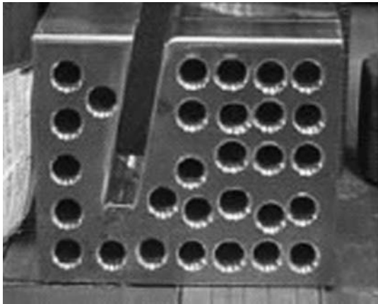
FIGURE 3.19 After: A 45% reduction in the weight of the forming blocks was achieved by carefully adding lightening holes to the blocks. (From Boeing Commercial Airplane Group Seattle, WA 2003 and Zawitz Ben, Ergonomics at Boeing . Ergosolutions magazine July/August 2003. With permission.)
