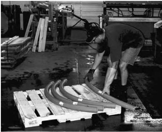
FIGURE 3.20 Palletizing PVC pipes required repetitive bending of the back several hundred times during the work shift.
