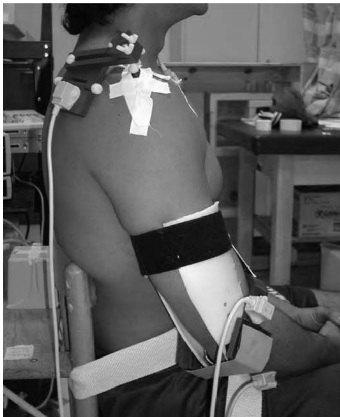
FIGURE 10.5 An electromagnetic system being used to measure shoulder and upper extremity motions. (Courtesy of Richard Hughes, University of Michigan Orthopaedic Surgery Department. With permission.)
