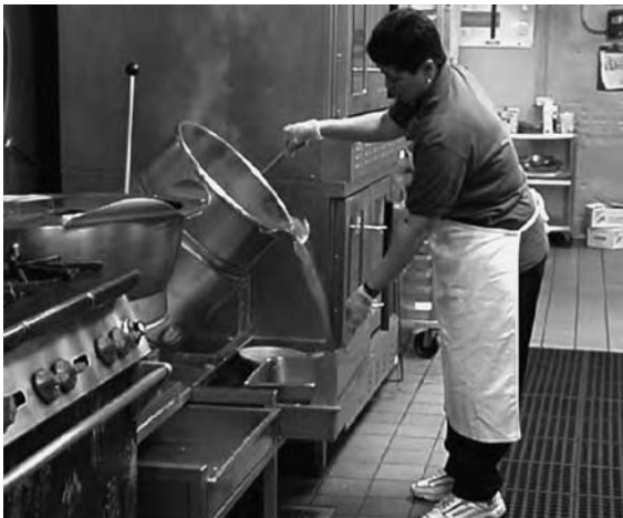
FIGURE 3.15 A tilting soup pot allows for easier soup dispensing in dietary services.
