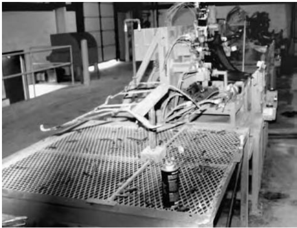
FIGURE 16.28 An adjustable frame for mounting a unit on which work is to be done is set toward the working edge. The reach for the unit is reduced and the unit does not need holding while work is performed.
