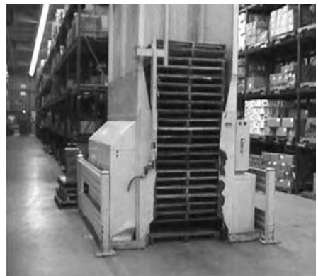
FIGURE 45.20 Wooden pallet dispenser used to reduce the manual handling of pallets.
