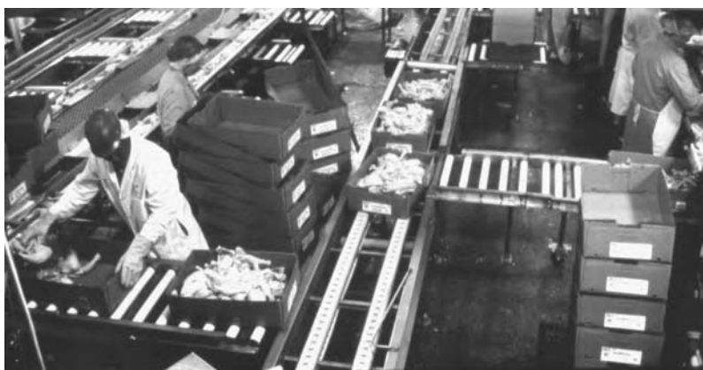
FIGURE 16.6 Filled boxes are pushed across connecting roller conveyors onto the central shipping line.
