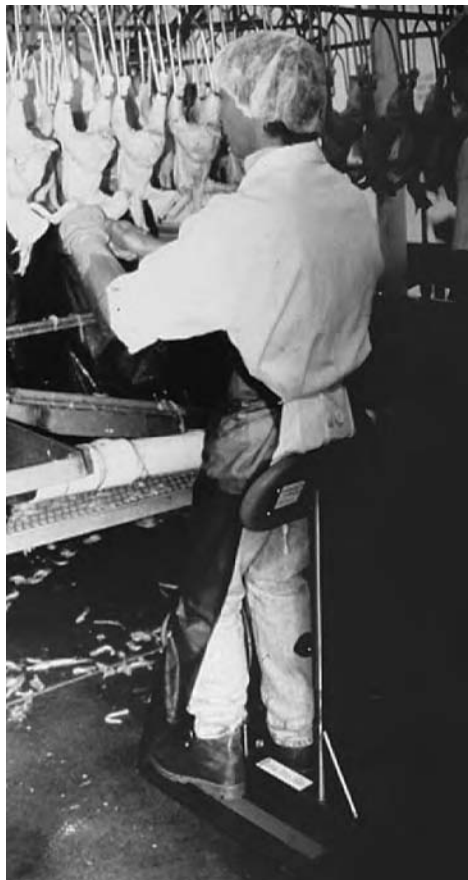
FIGURE 16.30 A lean stool that also has knee support. The stool is alternated with standing rather than used for a whole shift.
