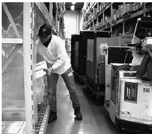
FIGURE 3.11 After: The stored boxes were raised to a more comfortable lifting height to reduce awkward lifting postures.
