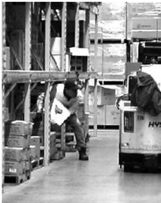
FIGURE 3.10 Before: Boxes of products used to be stored on pallets on the ground, requiring back bending to lift and handle the boxes.
