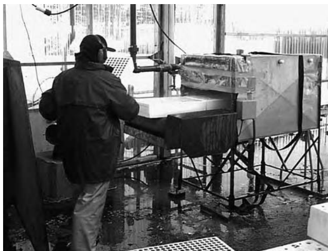
FIGURE 3.7 After: An automated block washing system to reduce physical risk factors and increase productivity.
