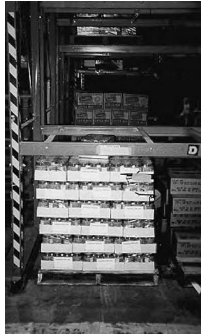
FIGURE 45.11 Tight fit of a pallet in a half slot, making some cases difficult to retrieve and requiring selectors to bend or reach excessively.
