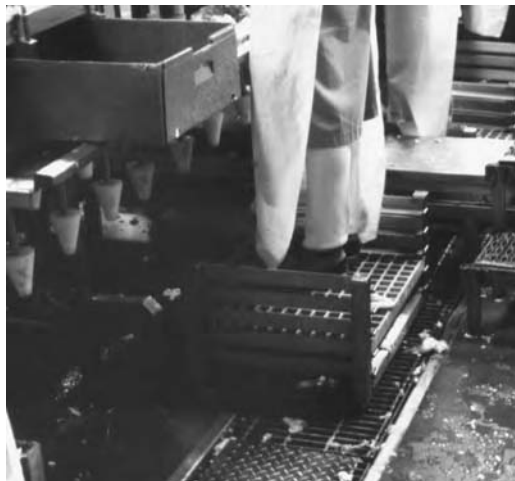
FIGURE 16.25 Adjustable work platforms raise the height of the worker.
