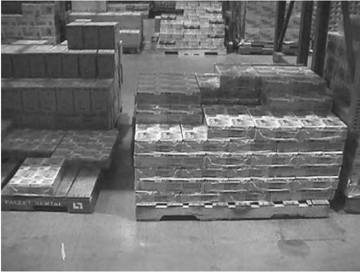
FIGURE 45.19 Pallets set apart in a slot to increase the clearance between pallets and provide easier access to selectors.
