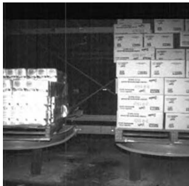
FIGURE 45.5 Raising pallets off the floor by using risers in a full slot.
