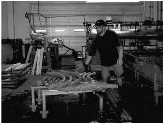
FIGURE 3.21 The ergonomics committee designed this knee-height cart to reduce bending of the back.
