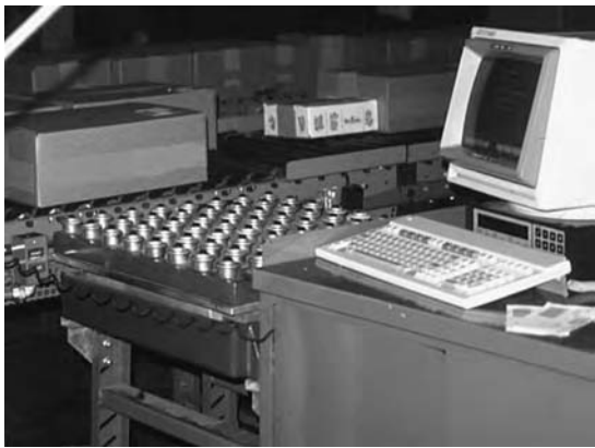
FIGURE 16.27 A connecting table with multidirectional rollers provides an easy method to pull and push product on and off line. The table is integrated with scales.
