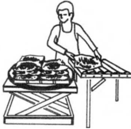
FIGURE 11.7 Turntables can be rotated to reduce reaches and moves by the operator. One option is to mount the turntable on the floor and place a pallet on it. The turntable (as well as ball casters and air-film tables) also can be mounted at a fixed height (such as even with a conveyor or worksurface). A scissors lift moves up and down to reduce lifting/lowering stress. If it is at the height of the work, the work can be transferred to/from it with a sliding motion instead of lifting/lowering. Of course, a scissors lift can be combined with a turntable. (From Hanna, S. and Konz, S. 2004. Facility Design and Engineering , 3rd ed., Holcomb Hathaway, Scottsdale, AZ. With permission.)
