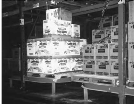
FIGURE 16.9 The pallet racks are permanently raised off the ground so that the hand height to lift the lowest case is between the hips and shoulders.
