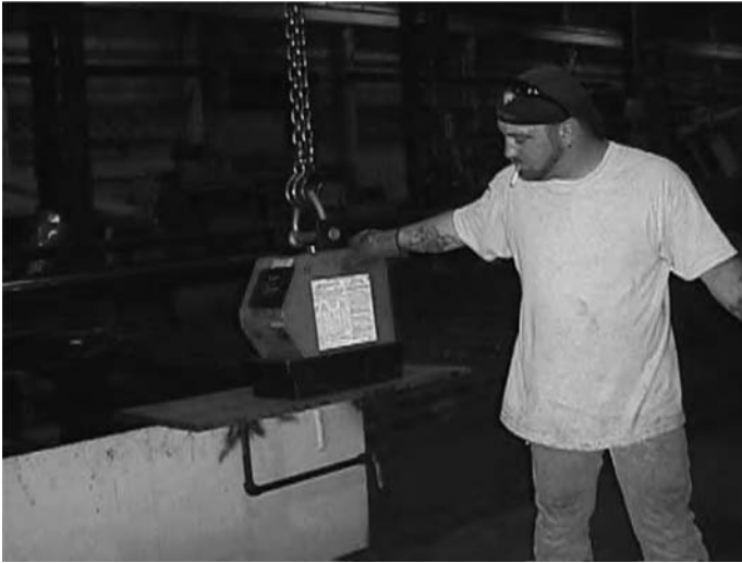
FIGURE 13.4 Magnetic lift attached to a hoist.
