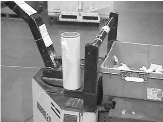
FIGURE 45.22 Example of holder on a pallet jack to secure plastic-wrap rolls.
