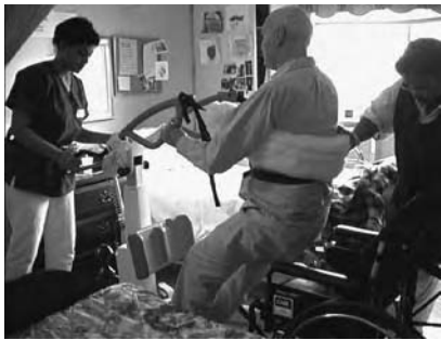
FIGURE 3.14 A sit-to-stand lift for partially weight-bearing residents to control lifting hazards.
