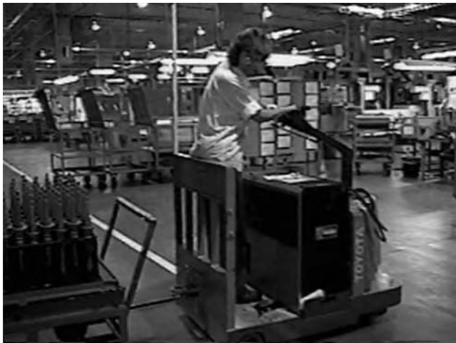
FIGURE 13.5 Tug being used to pull carts, eliminating the forces associated with manual pushing and pulling.
