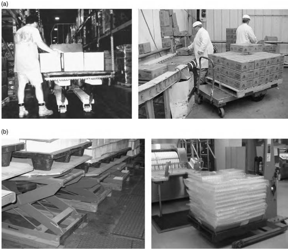
FIGURE 16.10 (a) Two illustrations show the pallet raised for loading. The picture on the left hand side in a distribution center shows the forks of a pallet jack raised up so that the first few layers of the pallet are stacked at around waist height. The picture on the right-hand side shows a simple platform truck being used to raise the pallet for palletizing from the conveyor belt. The platform truck reduced deep bending and more women were able to perform the job as the forces were reduced. (b) Two illustrations show the pallet raised up for unloading. The picture on the left-hand side shows traditional scissor lift tables that raise the pallets of paper, which are removed during the job. The picture on the right-hand side shows a forklift being used to raise the pallet for unloading.
