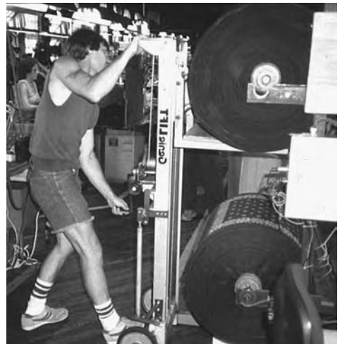
FIGURE 16.4 An employee is using a small mechanical lift to raise a roll of material to mount onto a machine.
