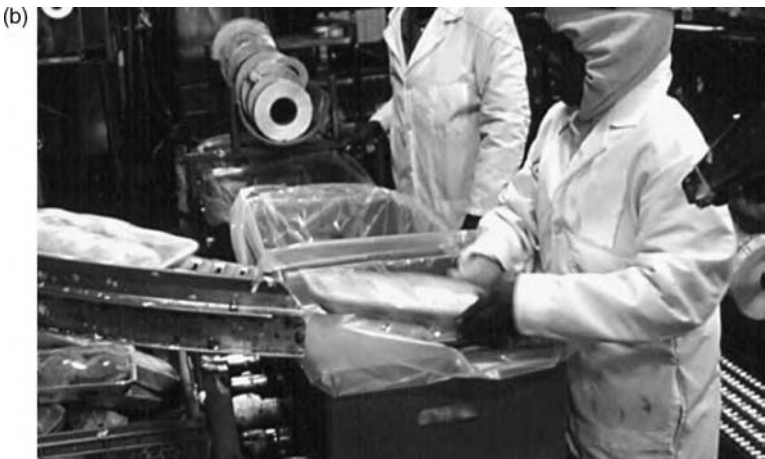
FIGURE 16.8 (a) Each packet of product is picked up by the left hand and passed to the right, which then stretches to place the product into the box. (b) Gravity brings each packet down a nonpowered roller conveyor to the box. The employee guides the product, letting it fall into position.
