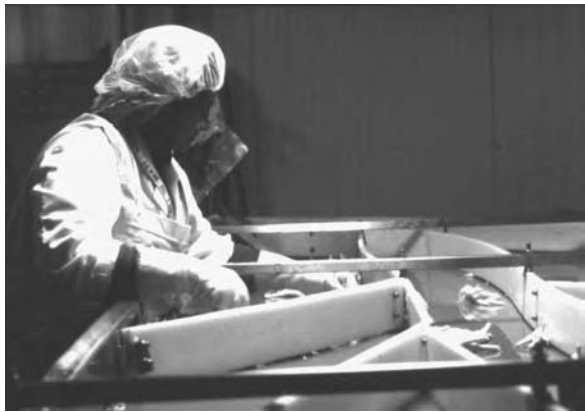
FIGURE 16.26 Diverters direct the work close to worker so that reaching is prevented.
