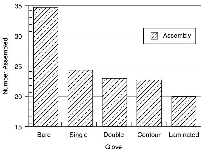
FIGURE 18.4 Glove effect on assembly time.
