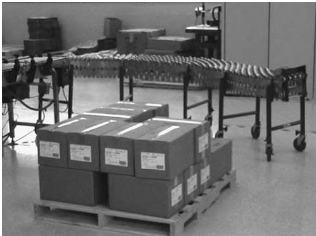
FIGURE 16.22 Flex conveyor in position to bring cases closer for palletizing.
