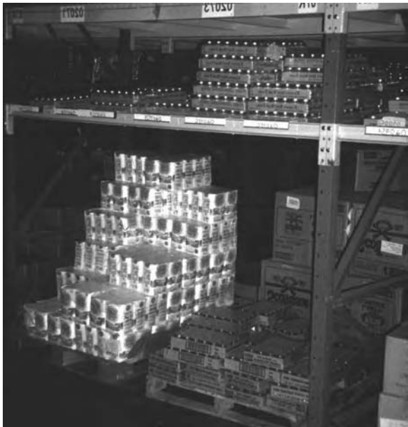
FIGURE 45.14 Gravity-fed flow racks used above a near-full slot.
