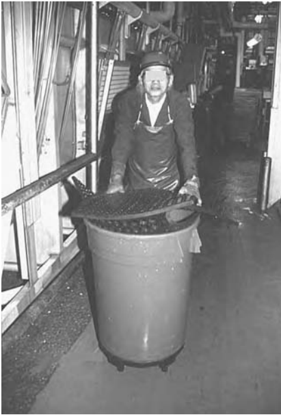
FIGURE 16.21 Pushing a barrel on a dolly. Note the broken handle that occurred when pulling the barrel without a dolly.
