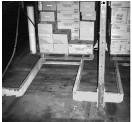
FIGURE 45.16 Risers used to elevate pallet from the floor and allow easier access to cases, but may create a tripping hazard.
