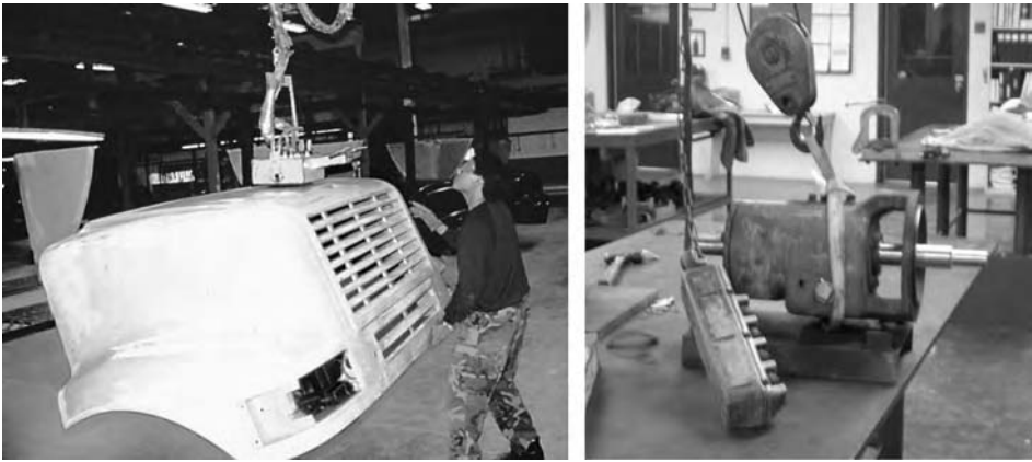
FIGURE 16.3 Two examples of hoists: one on the left is a vacuum hoist and the other on the right is a simple chain and strap hoist.
