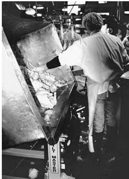
FIGURE 16.14 The product is tilted so that it is closer to pick up. A tank tilter such as this also raises the product to waist height. The reduction in fatigue on the worker improves the performance of unloading the tank.
