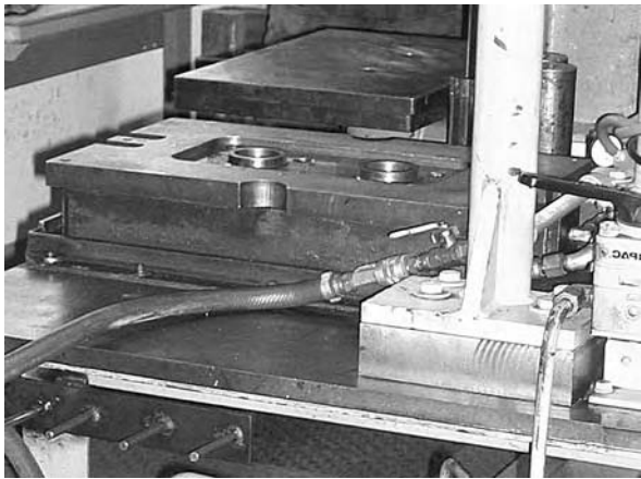
FIGURE 16.7 An air system (note air hose to fixture) floats the heavy base of a unit so that it can be manually pushed with ease, into position under the press.
