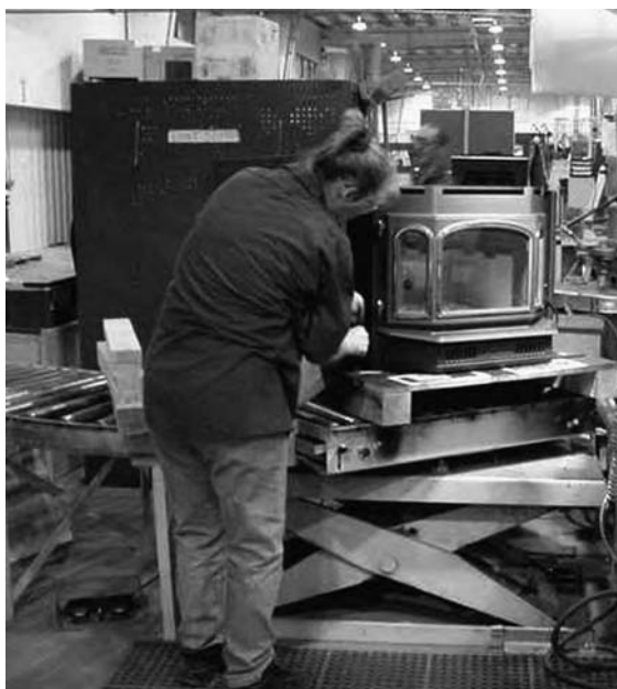
FIGURE 3.3 Scissors lift tables with rotating tops allow height adjustability for the worker, and prevention of neck and back awkward postures.
