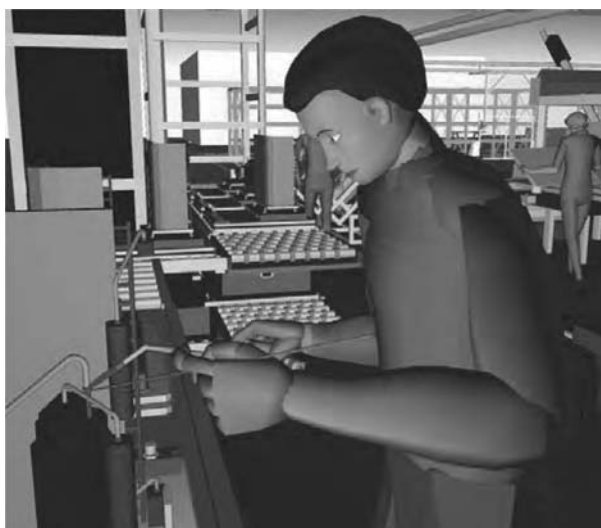
FIGURE 10.1 A digital human figure model in a virtual manufacturing workstation rendered by Jack for static reach, fit, and visibility assessment. (Courtesy of Ulrich Raschke, UGC-PLM Solutions. With permission.)
