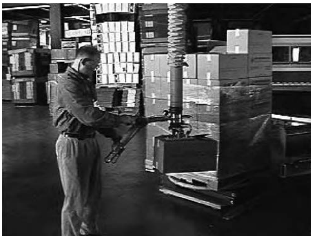
FIGURE 13.3 Vacuum lifter being used to lift a load.
