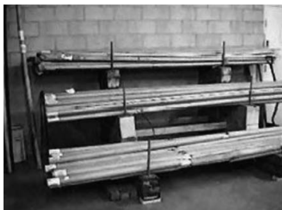
FIGURE 3.24 Vertical stacking of material was replaced with horizontal stacking that allows forklifts to do more material handling.
