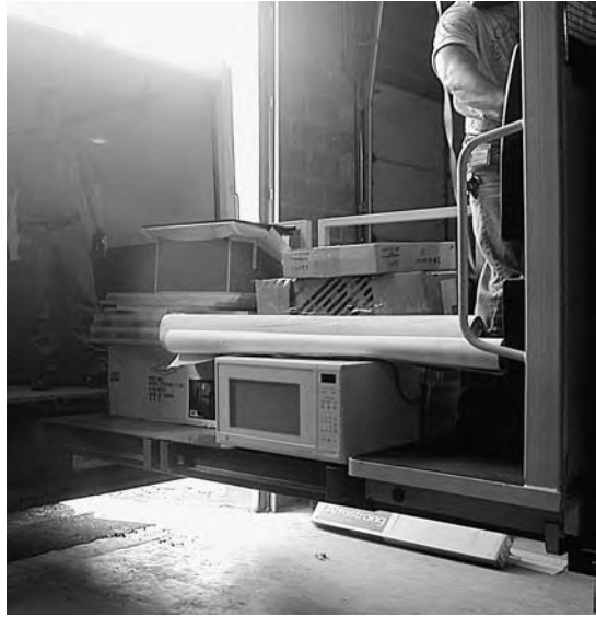
FIGURE 16.13 A platform lift takes the operator up above the floor to the height of the truck for unloading.
