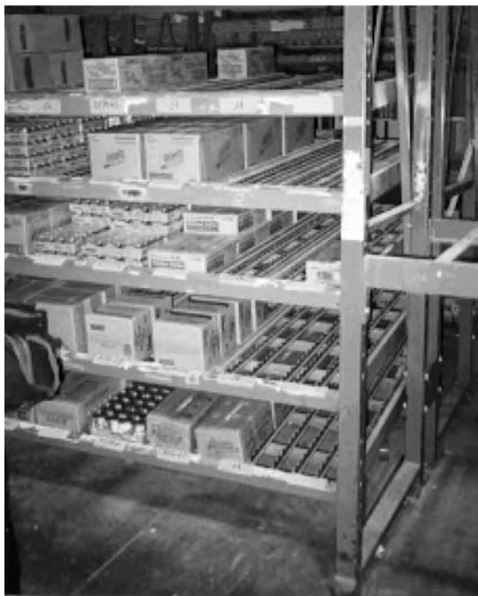
FIGURE 45.15 Gravity-fed flow racks.
