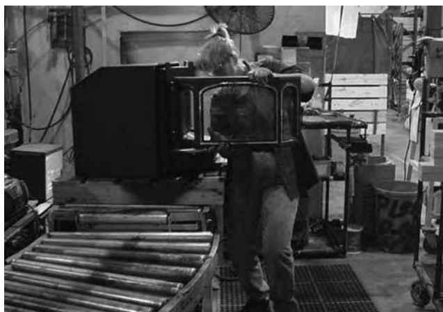
FIGURE 3.4 Roller conveyors on the assembly line eliminate lifting heavy parts.
